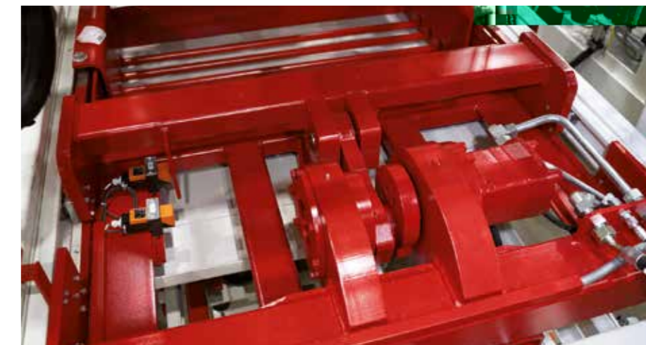
Hydraulically driven filler grid, for optimized filling of the mold and cycle time reduction
